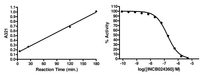
IDO1 activity (right) and IDO1 inhibition (left), measured using the IDO1 Inhibitor Screening Assay Kit, BPS Bioscience, Catalog #72034. *Data shown is lot-specific. For lot-specific information, please contact BPS Bioscience, Inc. at info@bpsbioscience.com*.
