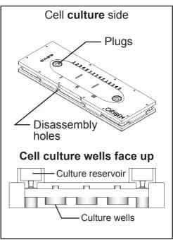
The CellGem® chip consists of 3 different layers shown in below.
