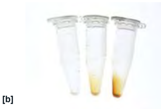
Fig. 6 (a) The precipitation of \alpha -elastin (0, 25 & 100 \mu g) following the addition of the Elastin Precipitation Reagent. (b) Dye bound \alpha -elastin (0, 12.5 & 25 \mu g) after removal of unbound dye from the tubes.
