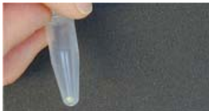
[1] Cold precipitated elastin, ( 1 mg ), overnight, then centrifuged and drain dried
