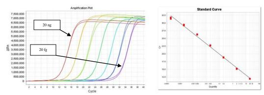
**Reliable standards for the quantification of human DNA:** Human DNA Standards (measured in duplicates) comprise a 10-fold dilution series ranging from 20 ng to 20 fg.
