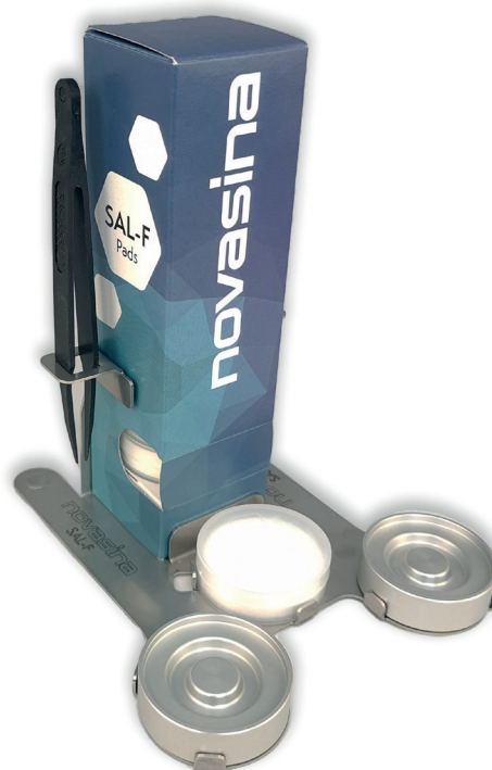
Figure 3. Novasina SAL-F StarterKit which contains a holder, two aluminum cups, tweezers and one box of SAL-F Pads. The StarterKit with the new SAL-F standards allows the fastest possible calibration and verification.
