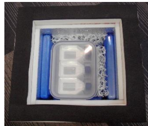
Place the second secondary container set on top of it. Fix the secondary container with 2 mesh cushions.
